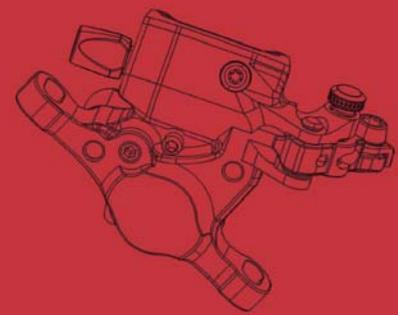
The HYRD brake system is an open hydraulic brake designed for use on single rider bicycles. The purpose of the open hydraulic system is to allow the pistons to compensate for pad wear. Each time the brake is released, the piston opens up the reservoir, allowing more oil into the caliper if needed. Only a properly set-up brake will allow the piston to retract fully ensuring that your brakes can account for worn pads.
