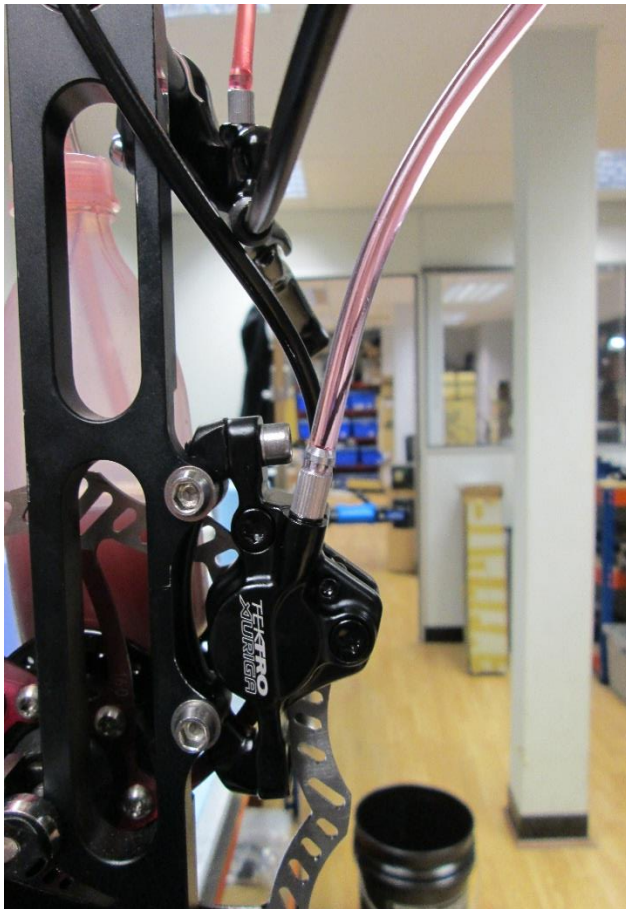
Attach syringe of oil to the calliper bleed port.
