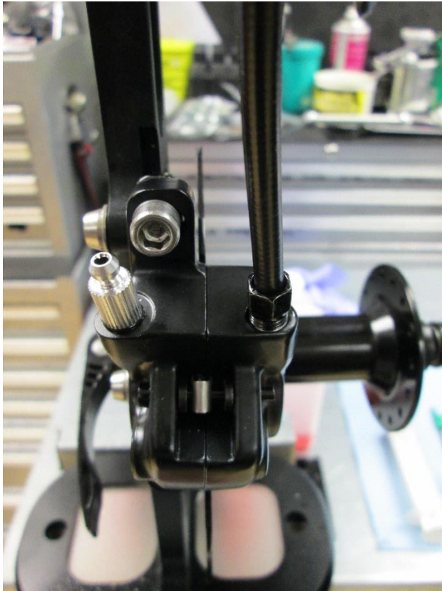
Insert second Tektro bleed nipple.
