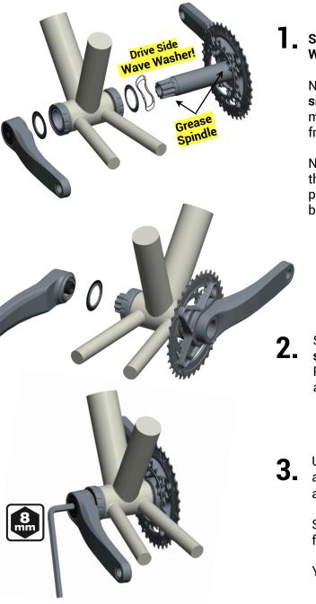
Slide the Drive side 30mm ID Wave Washer onto the spindle.
