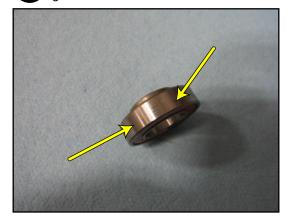
It is best to use alcohol to clean bearings, bearing pockets, and threads to ensure no oil or grease is on any of the surfaces during the assembly process
