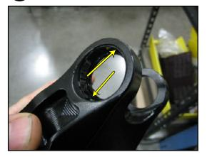
Before installation clean oil and grease off of bearings and link.
