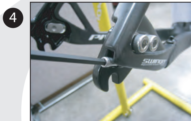
Use 4mm hex key to adjust chain tension. Count indexed "clicks" on each side to match DS/NDS dropout distance.
