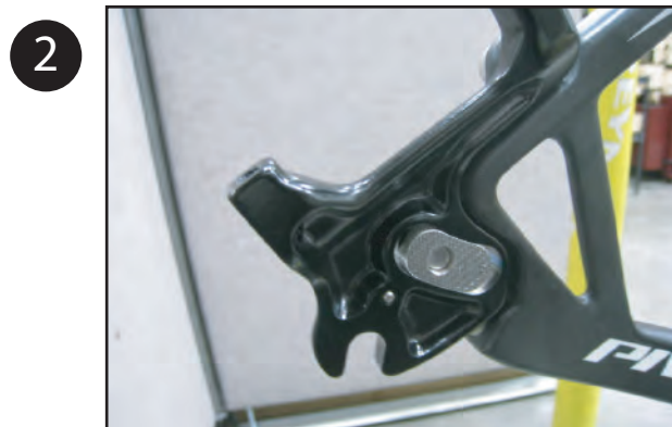
NDS dropout installed like image. Flip nut 180 degrees to extend travel.
