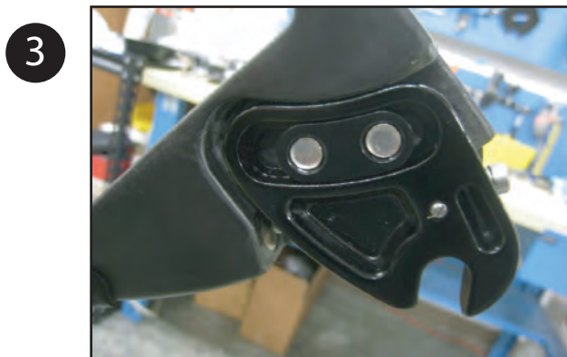
DS dropout installed.
