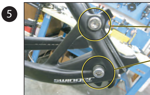
Torque bolts as shown. Use Blue Loctite.
