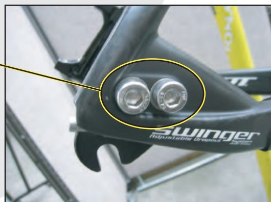
Use 4mm hex key to adjust chain tension. Count indexed "clicks" on each side to match DS/NDS dropout distance.
