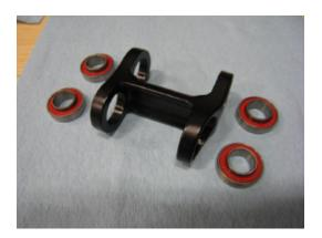
Bearing race must be clean of oil or grease
