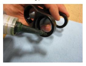
Use a toothpick to spread the Loctite to coat bearing pocket
