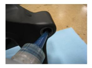
Use a toothpick to spread the Loctite on threads
