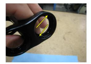
8 Apply Loctite 242 or 243 to threads in frame
