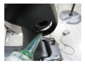
Use a toothpick to spread the Loctite to coat threads
