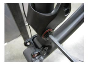
Apply Loctite 609 or equivalent to NDS bearing pocket
