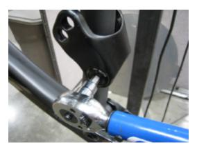
Check motion of link to ensure free movement
