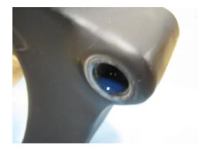
Use a toothpick to spread the Loctite on bearing pocket
