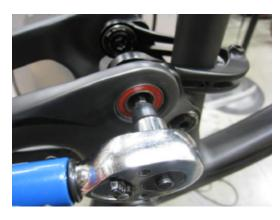
Torque bolts to 35Nm
