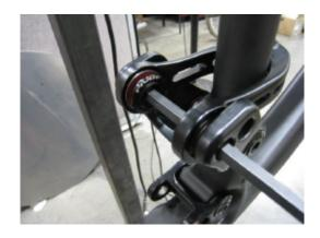
Torque bolts to 35Nm
