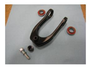
Apply Loctite 609 or equivalent to DS bearing pocket only
