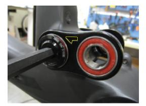
Torque bolts to 35Nm
