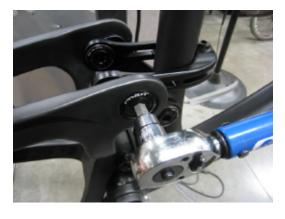
Torque bolts to 35Nm
