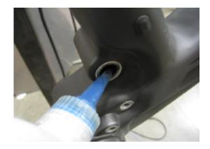
Use a toothpick to spread the Loctite to coat threads
