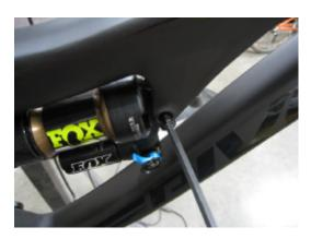
Torque clevis bolt to 32Nm
