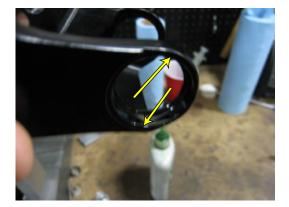
Before installation clean oil and grease off of bearings and link.
