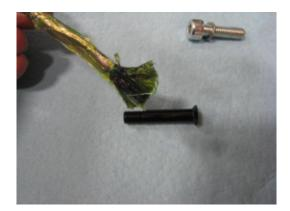
Torque shock tab bolt to 13Nm
