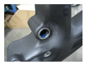
**10 DO NOT** apply Loctite on bolt threads
