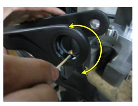
Apply Loctite 242 or 243 to RT threads on both sides
