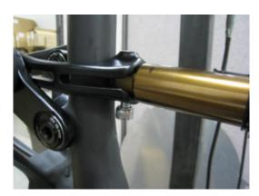
Once frame is cleared, align shock vertically in tabs
