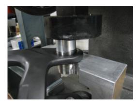
Use enough Loctite to cover threads as shown
