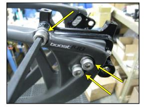
Adjust dropout until bottomed out in the forward position
