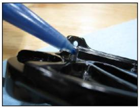
2 Install detent screw about two threads in by hand
