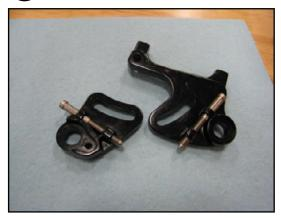
9 Install dropout lock nuts
