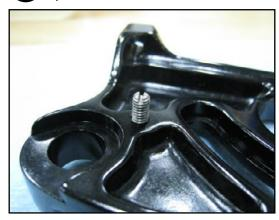
There should be no excess Loctite – only cover upper portion of threads
