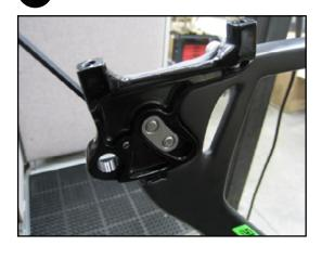
When adjusting chain tension/wheel position, it is recommended to start in the full forward position, and count clicks out as a reference between DS and NDS adjustment.
