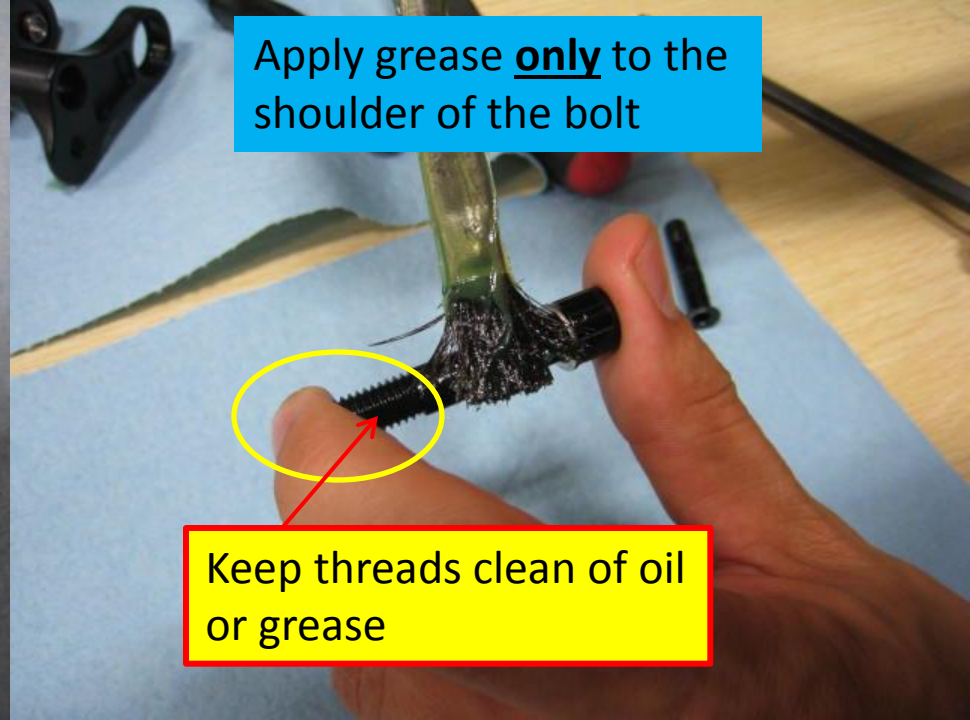
Apply grease or anti seize to shock bolt
