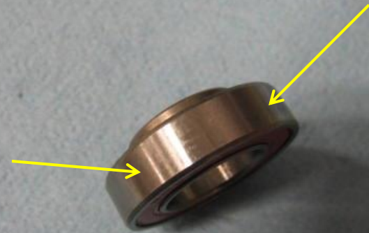
Bearing race must be clean of oil or grease
