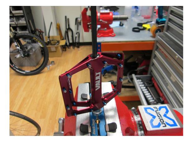
After fitting the end cap, spin the axle and see if it has excessive drag. If so, the axle may need a light sanding to get rid of any stubborn bushing staining.
