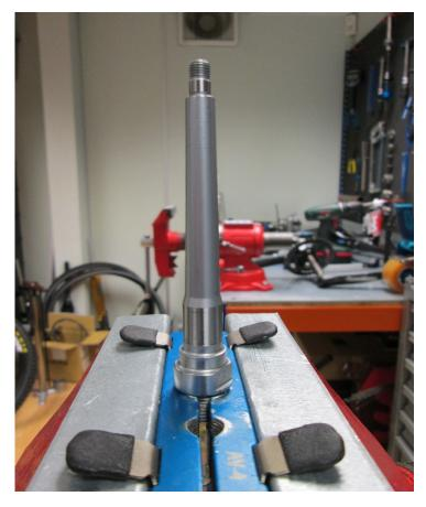
Remove the old rubber seal and clean the axle of any old dirt and grime and inspect for any imperfections on the bearing surfaces.
