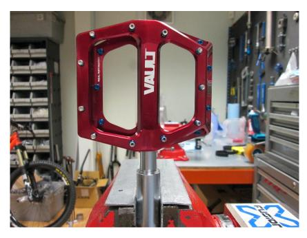
Making sure the body is clean of all dirt & debris, square the body up to the bushing and push with your hands until it stops.
