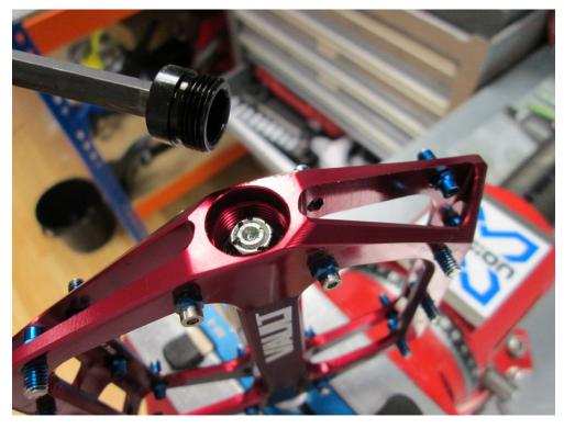
Hold the pedal axle using the a 6mm hex key.
