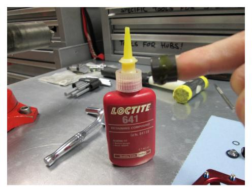
Use a dab of Loctite 641 to make sure the bushing doesn't ride out of the pedal body in the future. Slide the new bushing onto the tool ready to be pushed into the pedal body. Notice that one end of the bushing has a slight chamfered edge, that enters the pedal first.
