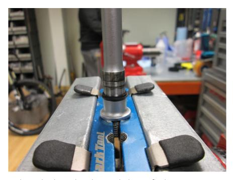
Slide the new rubber seal onto the clean axle and grease the bearing/bushing contact points ready for the pedal to be re-assembled.
