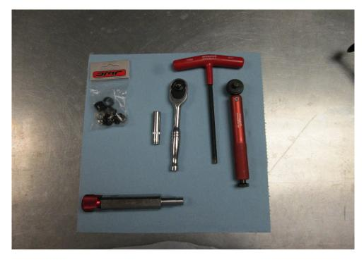
**Tools Needed:** 2 x 6mm hex Key, DMR Vault & V12 Tool, ¼" Ratchet with 8mm Socket, ¼" Torque Wrench **Parts Needed:** DMR Vault Service Kit.
