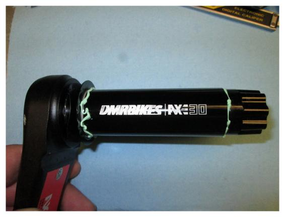
After the bearings have been pressed into the frame it's time to prep the crank. Slide the wavy washer on to the axle followed by the dust cover, and apply a small bead of water resistant grease.
