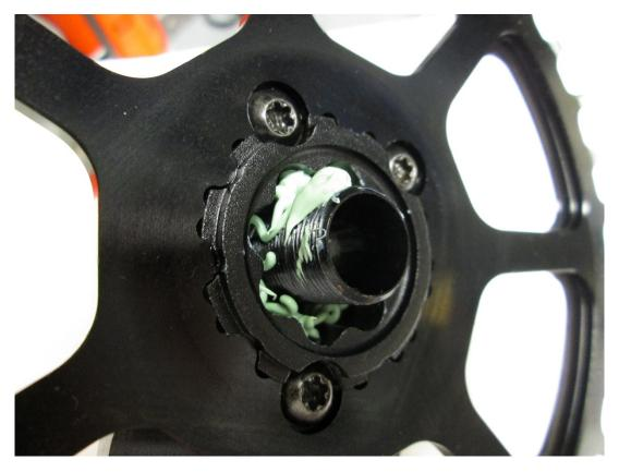
Grease the spline on the inside of the crank arm making sure you also grease the bolt threads.
