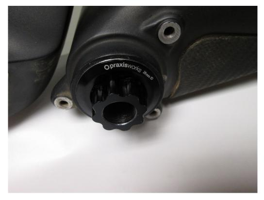
Slide the crank into the frame so the splines slightly protrude through the drive side (28mm Bearing).
