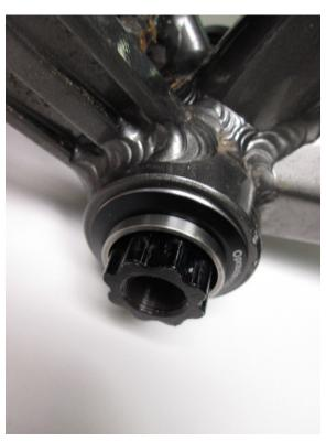
Finally, Torque the arm onto the axle to 48-55Nm and check your chain ring clearance and crank arm clearance. They will be even on each side. If you have a seat tube that is designed to be off centre to make room for linkages for example it may prove to be difficult to get an accurate chain line measurement, but try your best to find the frames centreline and measure outward toward the chain ring teeth.
