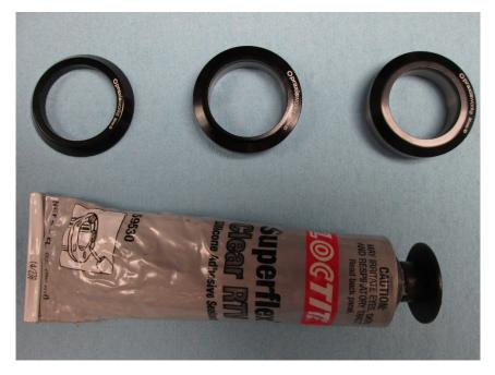
For Carbon frame applications you must use the Loctite Superflex RTV silicone bonding agent to assure that the bearings do not 'ride out' of the frame. The standard dust covers measure at 2mm and the thicker cover is 5mm.
