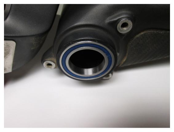
Press the bearings into the frame with a bearing press to assure the bearing is pressed in square and flat to the frame.
