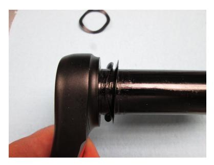
After you have pressed the bearings into the frame, go ahead and prep your axle as before. Slide the axle through the BB until the splines protrude through the drive side bearing.
