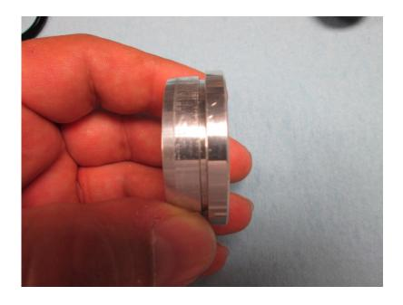
Apply only a small even coat around the entire outer race of the bearing as above. Before pressing the bearings into the frame, use the Praxis frame gauge (sold separately) to make sure your frame is within tolerance and not at any risk whilst fitting the bearings directly into the frame.
