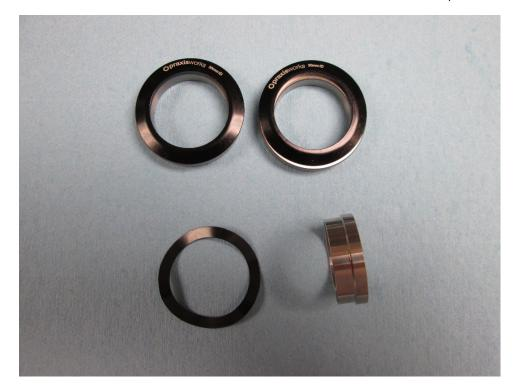
The difference being that the DMR BB has 2x 30mm ID bearings and proprietary axle position spacer.
