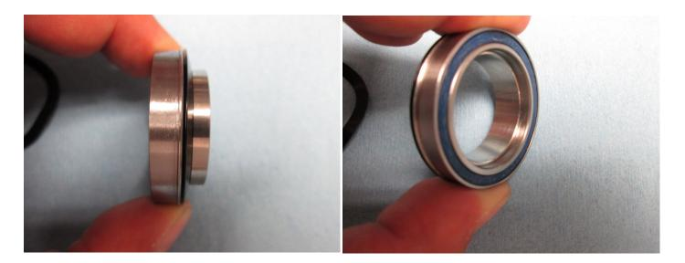
For Aluminium frames you NEED to use a Loctite retaining compound such as Loctite 638.
