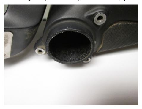
Start by cleaning the BB shell as good as possible with an alcohol based fluid to remove and past grease or oils, this is paramount in fitting our BB......
