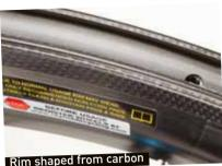
Reynolds going back to the lab to develop a new carbon/resin lay-up and expensive moulds in order to achieve the durability, strength and stiffness that was needed. It's also made the rims wider than most, which at 26.2mm at the widest point is pretty plump. This removes the 'balloon effect' caused by wide tyres on narrow rims, and as converts to running wider tyres it's hard to argue with that.
